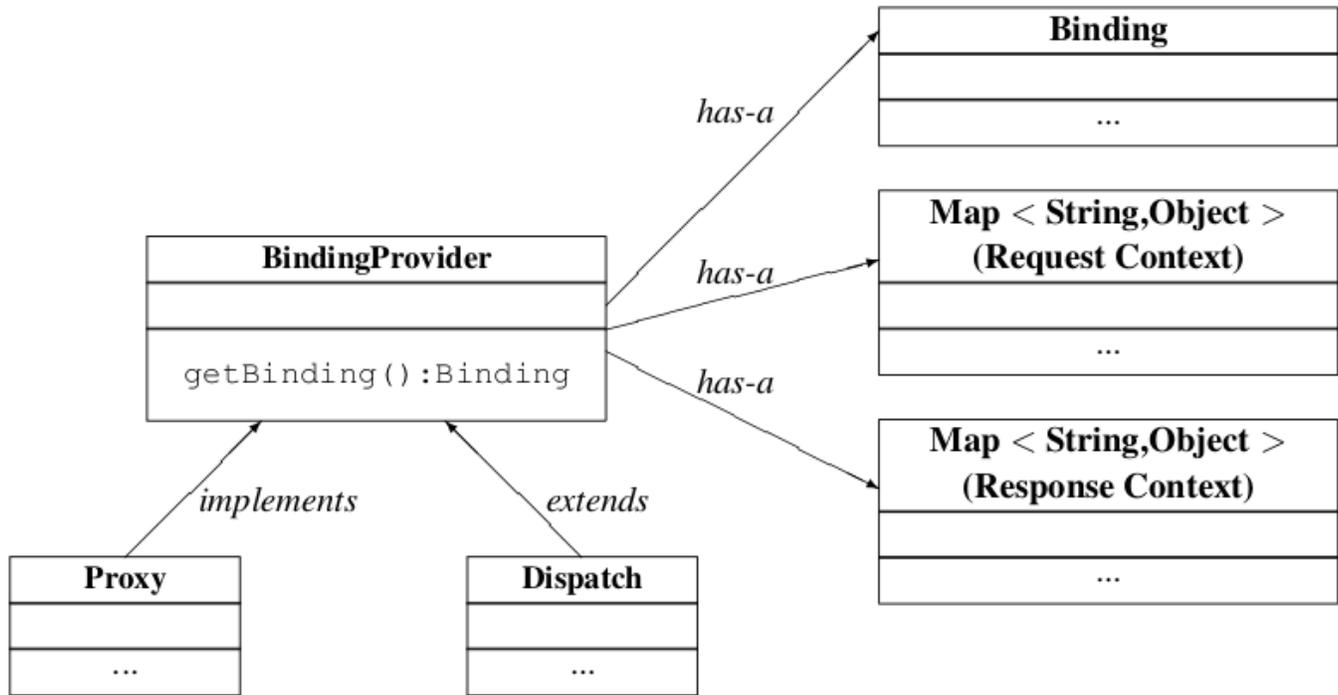
Figure 1. Binding Provider Class Relationships
