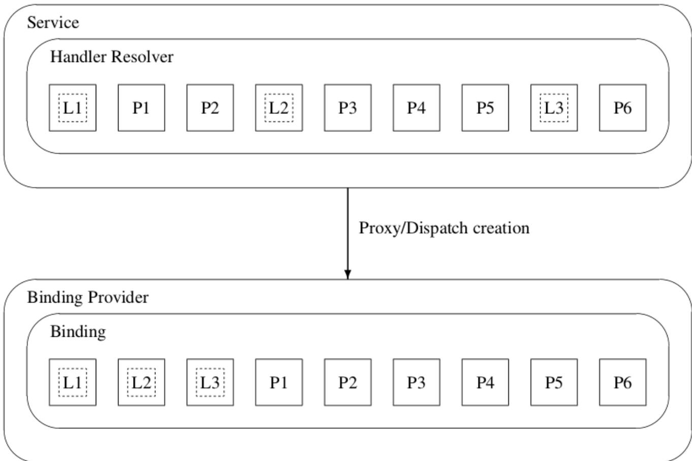
Figure 4. Handler ordering, Ln and Pn represent logical and protocol handlers respectively.
