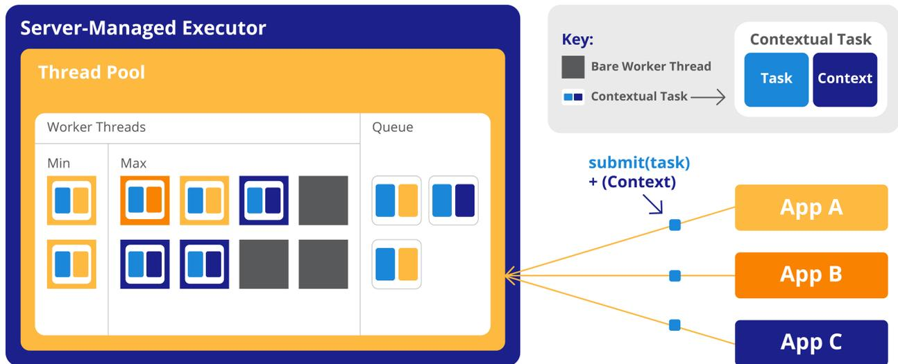
**Figure 3-1 Managed Thread Pool Executor Component Relationship**
