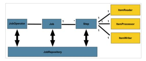
The diagram above highlights the key concepts that make up the domain language of batch. A Job has one to many steps, which has no more than one ItemReader, ItemProcessor, and ItemWriter. A job needs to be launched (JobOperator), and meta data about the currently running process needs to be stored (JobRepository).
