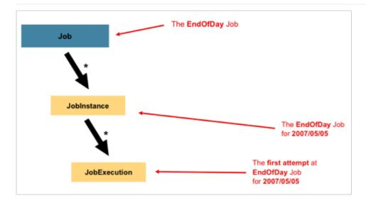
With Jakarta Batch, a Job is simply a container for Steps. It combines multiple steps that belong logically together in a flow and allows for configuration of properties global to all steps, such as restartability. The job configuration contains:
